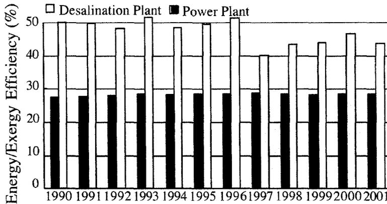
Fig. 2. Yearly energy/exergy efficiencies of power/desalination plants and conventional power-only plants of the utility sector, based on input and output energies and exergies in Saudi Arabia.
