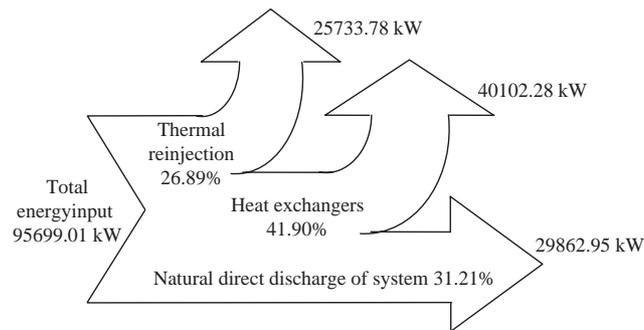
Fig. 2. Energy flow diagram (given as the percentages of brine energy input).
