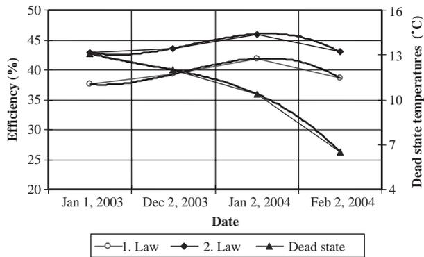
Fig. 7. Overall system efficiencies for different dead state temperatures.
