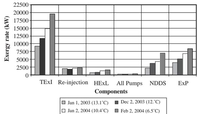
Fig. 6. Exergy flow chart in the graph of brine exergy input for different dead state temperatures.
