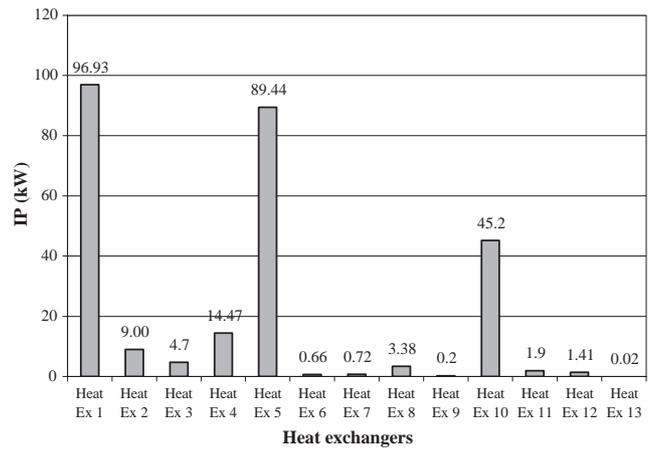
Fig. 4. Exergetic improvement potential of heat exchanger.
