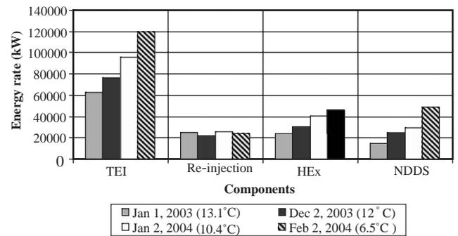
Fig. 5. Energy flow chart in the graph of brine energy input for different dead state temperatures.
