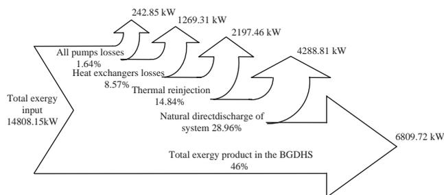
Fig. 3. Exergy flow diagram (given as the percentages of brine exergy input).
