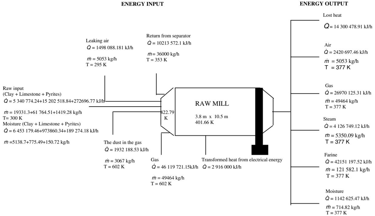
Fig. 4. Energy flow diagram of the raw mill.
