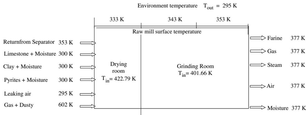
Fig. 2. Distribution of the temperatures in the raw mill.
