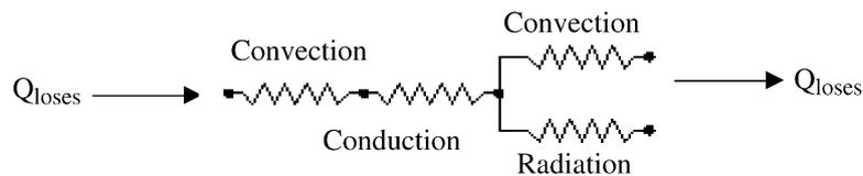
Fig. 3. Heat losses with electrical resemblance cycle.
