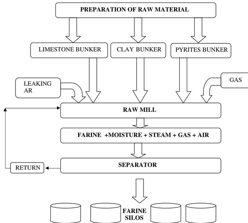
Fig. 1. Flow diagram of a cement plant process operation line.
